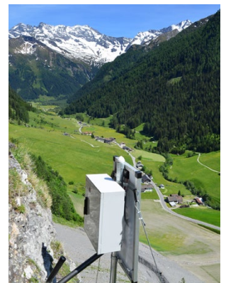
Monitoring mittels GPS (Vals)
